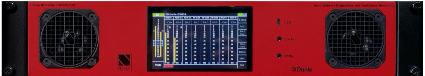
The front of the unit has a large 5" (127mm) Capacitive touchscreen TFT display plus two full range 63.5mm diameter speakers in optimally tuned and ported enclosures for confidence monitoring. The front panel is the location for the 3.5mm jack headphone output with mic input, the 3.5mm stereo line input jack and the USB micro AB connector for installing firmware updates.
