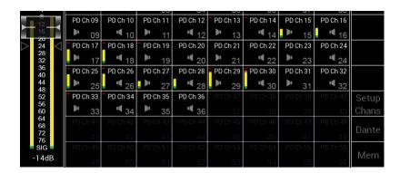
The Focus function on the RD Dante allows the user to highlight particular channels that are of more interest/importance
