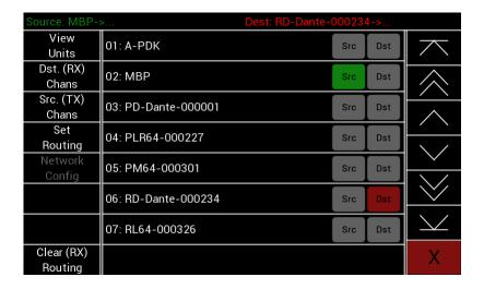
To set the routing between any pair of Dante devices attached on the same network. Press the Src (source) button for the device that audio is going to be listened too and it will turn green.
