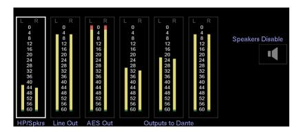
This page is split into seven areas, 6 stereo meters and a control area. Select an output by touching its meter. Controls for that output will then be displayed in the control area
